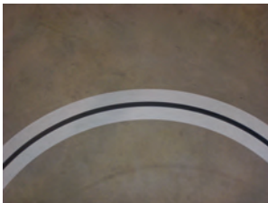
Sticker AGV track curve 90° b=160mm r=1m
